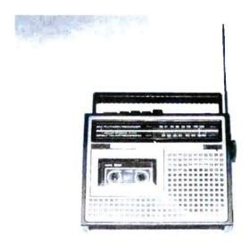
Amateurs and some professionals will typically use a standard tabletop portable radio with or without an automatic frequency conrol (AFC). Radios with standard analog tuning are required when the transmitter is not crystal controlled.
