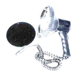
Spotlight with infrared lens. With the lens on, you cannot see any light with the naked eye. When you use it with a night vision scope, you can illuminate a suspect in a dark corner of a yard or an alley without his being aware that he is being observed.
