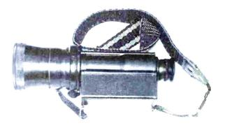
Surplus starlight night vision scope. It's great for spotting infrared light sources. You can see an infrared bug or an infrared remote control from more than a block away at night.
