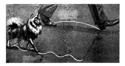
Fig. 24. WAVE-LENGTH AND FREQUENCY The length of a wave varies inversely with its frequency. The man's footsteps correspond to a frequency of 1 in relation to a frequency of 8 for the dog's.
