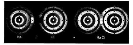
Fig. 20. CHEMICAL AFFINITY Atoms combine in order to fill vacancies in their outer orbits. Sodium, Na, combines with chlorine, Cl, and becomes common table salt, NaCl, because the sodium atom has in its outer orbit one electron, and the atom of chlorine has on its outer shell one gap to admit this electron.
