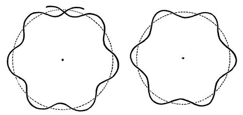
Fig. 47. THE MODERN CONCEPT OF THE ATOM The electrons swing along their orbits in "waves." The orbit of the electron can remain stable only if the oscillation of the wave corresponds to the length of the orbit. The pattern at the left is unstable.
