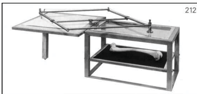
Rectangular dioptograph. Weight: 15.500 kg.
