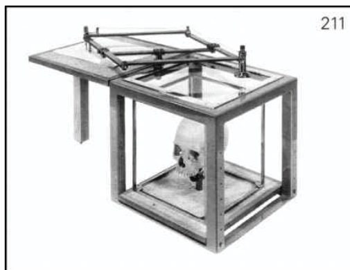
Quadratic dioptograph (Martin). Weight: 10.00 kg.
