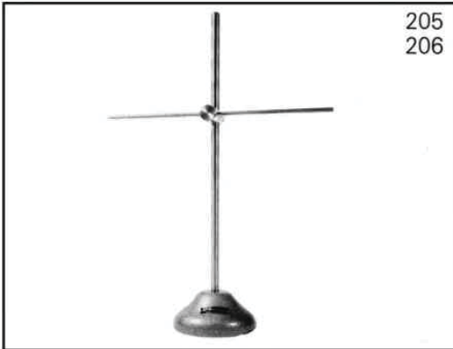
Left: Stylus for guiding horizontal lines. Height: 450-mm. Weight: 1.300 kg.
