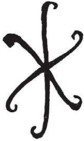
The "German man" as masonry anchor
