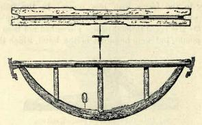
Fig. 426.—Rib of boat, showing seat attached
