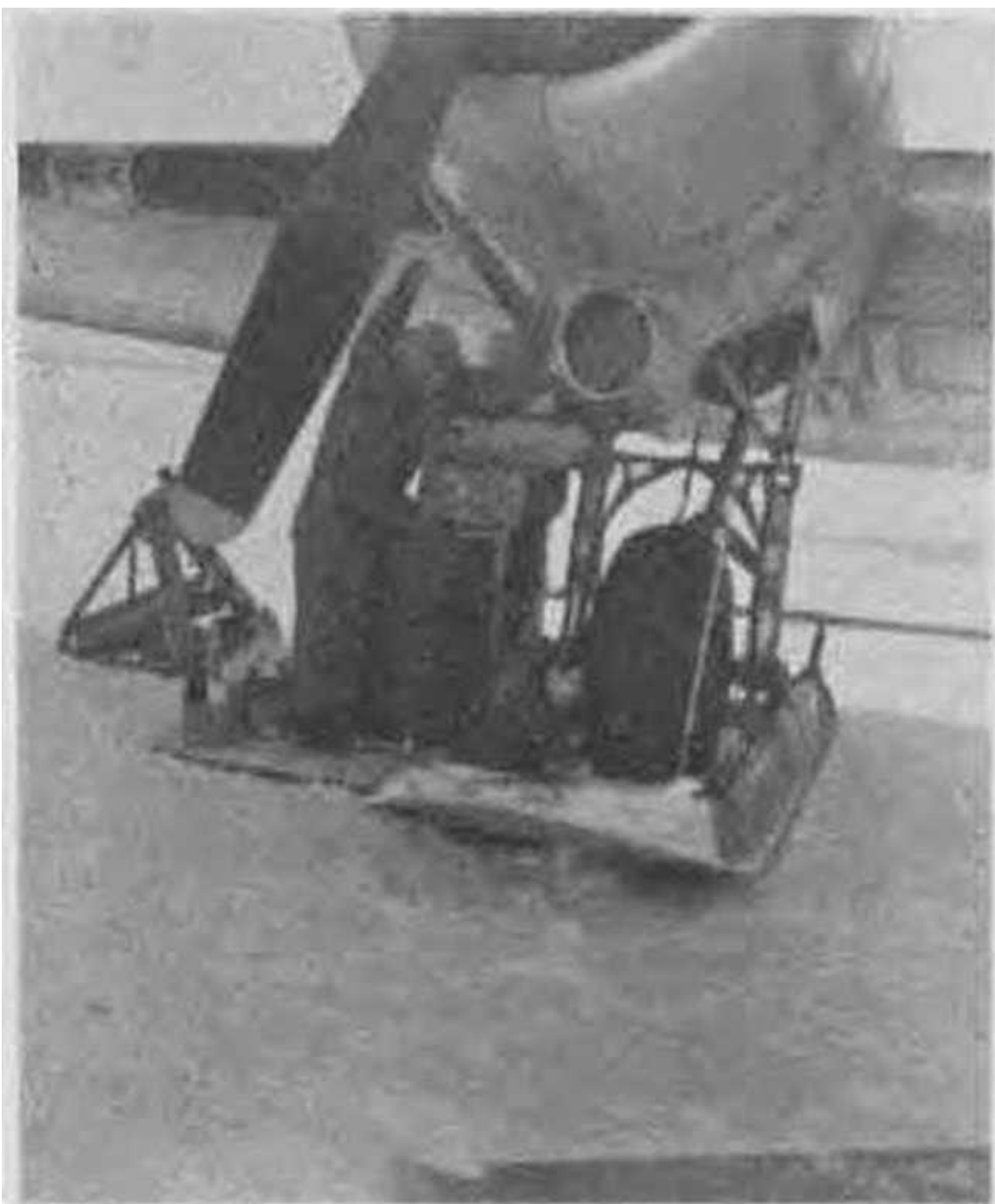
Figure 140. C-47 ski-wheel combination. Note cut out portion of ski surrounding wheel
