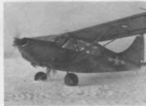
Figure 60. OY (L-5) stuck in newly compacted snow at end of PSP test strip.
