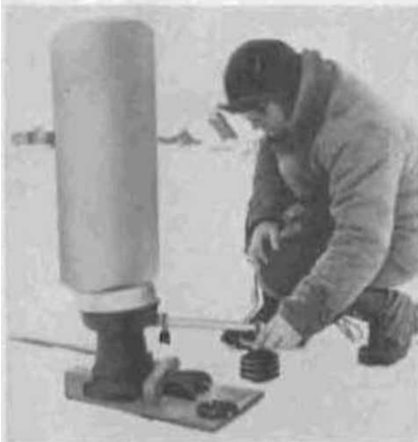
Figure 79. Weighing carefully measured specimen for density measurement.
