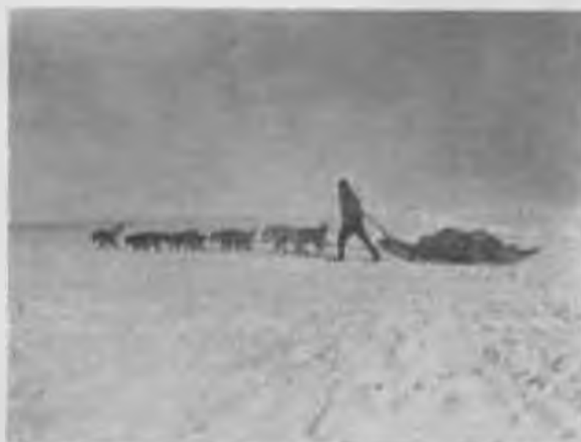
Figure 146. Dog team (nine dogs to team) showing cargo type sled with gee pole.
