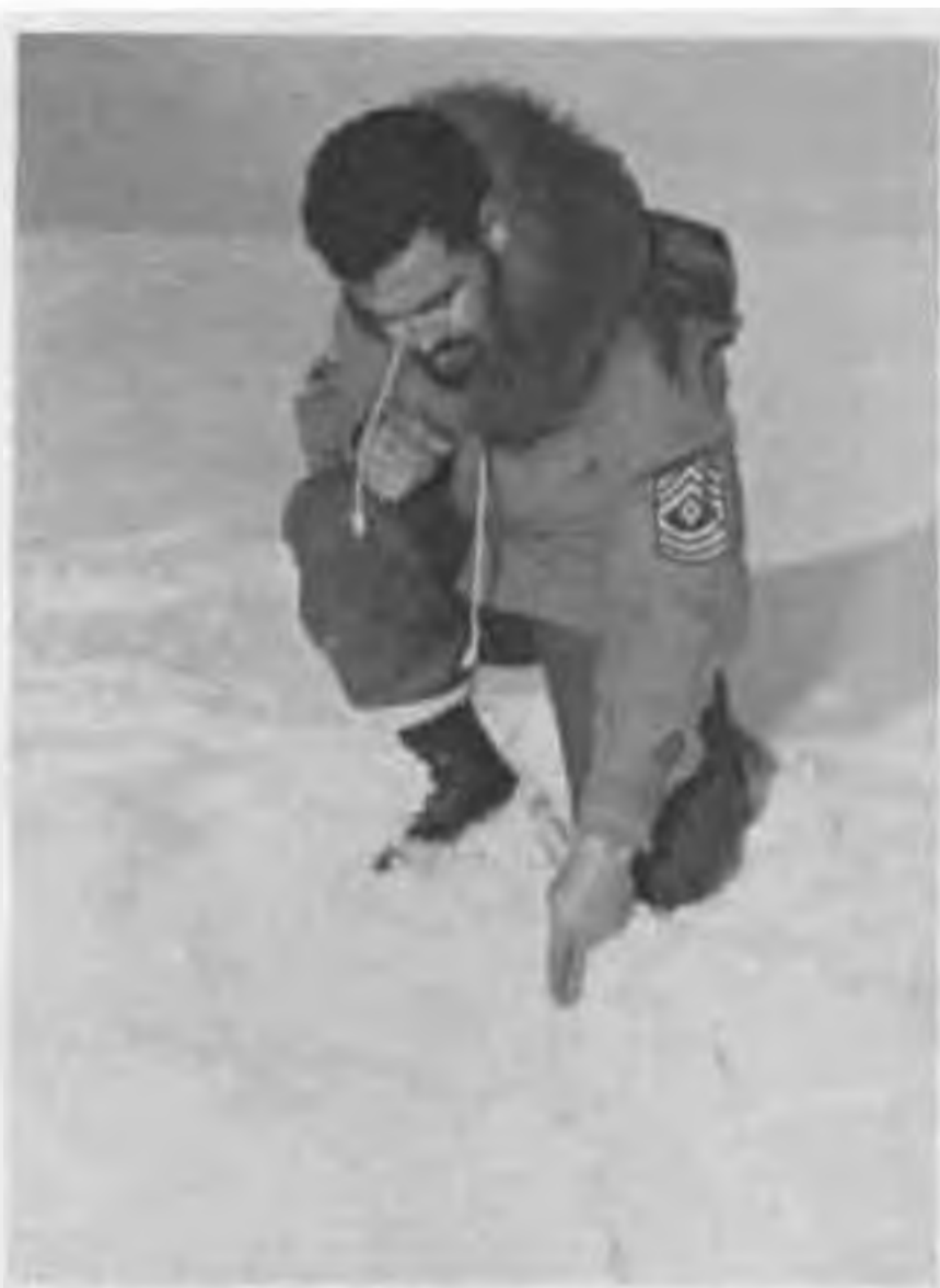
Figure 164. Sgt. S. A. London after parachute jump, showing depth of impact impression (approximately 2 inches).
