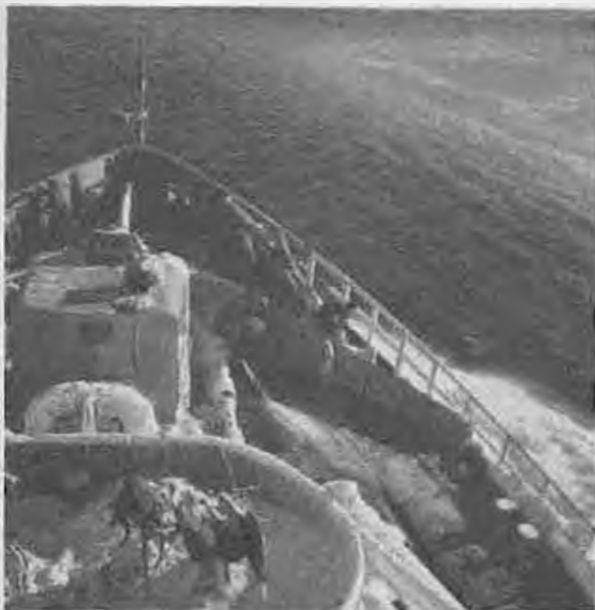
Figure 289. Spray ice, as found in the North Atlantic Ocean during winter months, formed on the U. S. S. Burton Island during a storm while the ship was en route to Little America IV.
