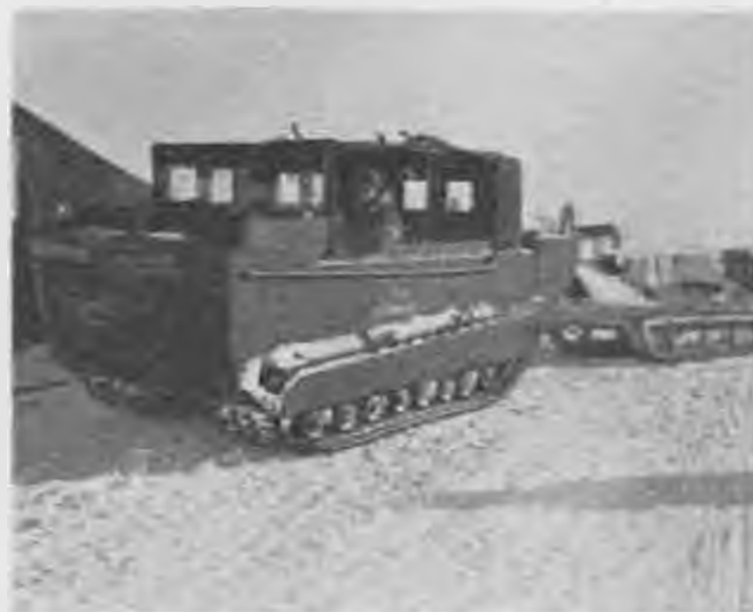
Figure 170. Vehicle assigned to dispensary showing quartermaster sled used for transporting crash equipment.
