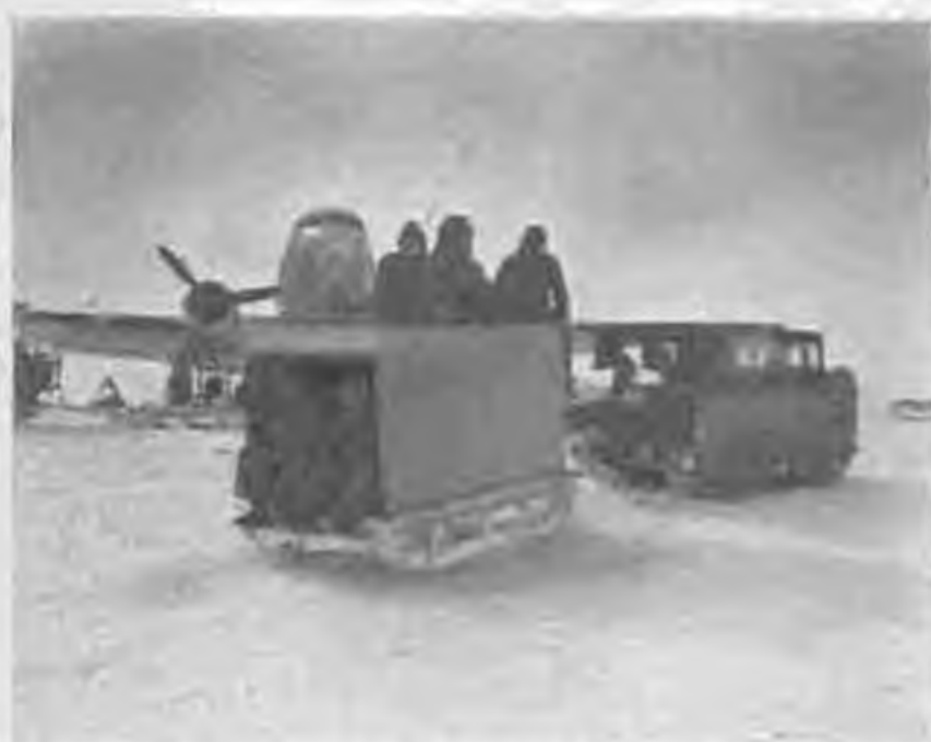
Figure 119. Box built on Army sled for personnel protection.
