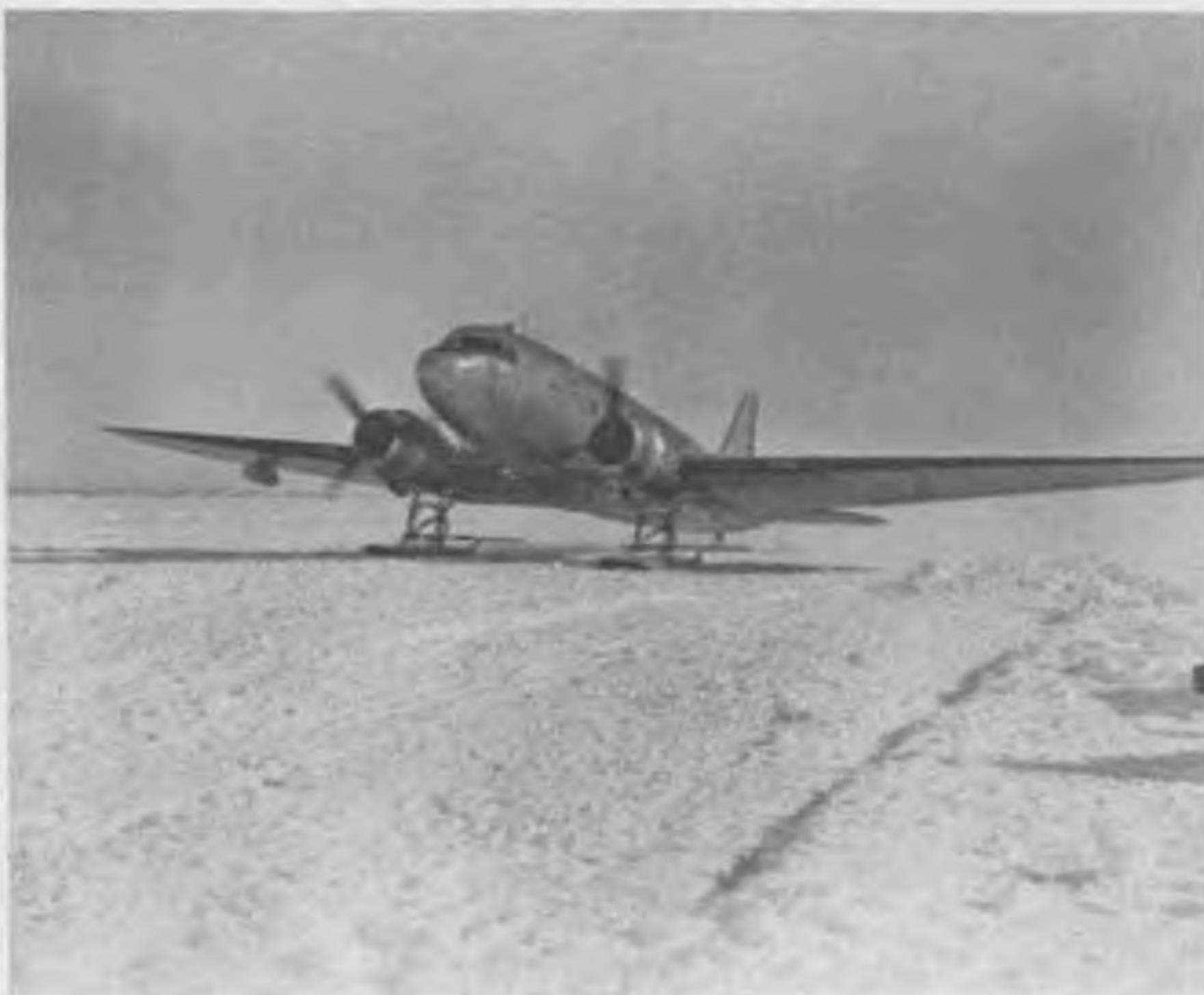
Figure 150. R4D (Army C-47) type aircraft on skis.
