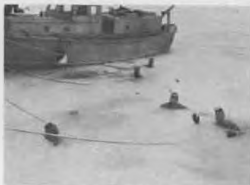
Figure 175. Immersion suits being tested. Note slush ice on surface of water.
