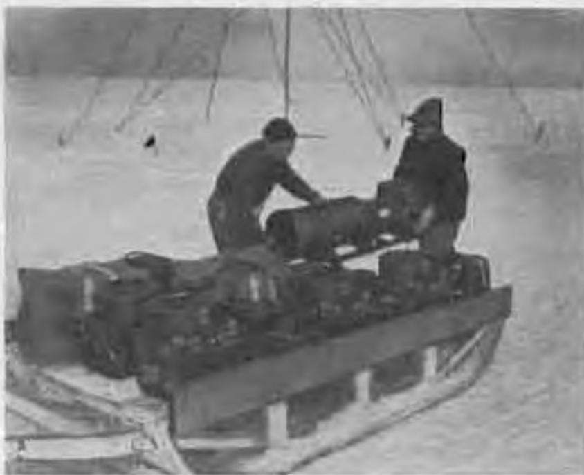
Figure 118. Sideboards added to Army sled keep airplane cameras from falling off in transit.
