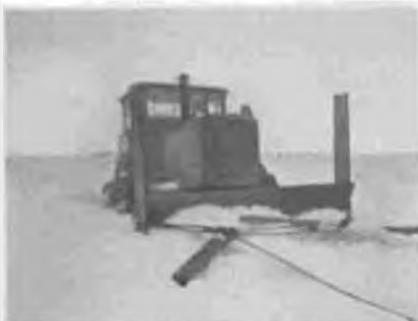
Figure 99. D-7 as "deadman" for hauling loaded sleds up barrier.
