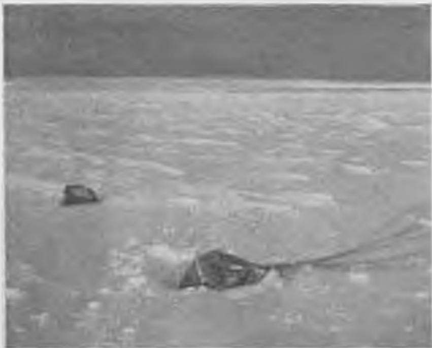
Figure 161. Results of unsuccessful aerial delivery cargo test, utilizing 24-foot Panatex Navy type quick attachable parachute. Cargo container buried itself 3 feet into hard snow (névé) surface. Parachute canopy did not open until unit was approximately 40 feet from surface.
