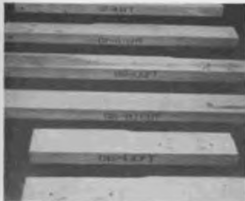
Figure 102. Layout of track extensions, showing both 60-inch and 30-inch types. D-6 tractors used only 30-inch extensions on Operation Highjump.
