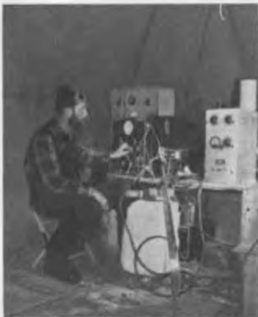
Figure 244. Sound attenuation measuring equipment.
