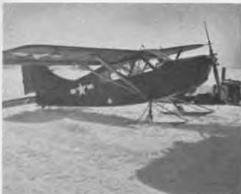
Figure 156. Army L-5 aircraft on skis. This aircraft was modified to carry one stretcher patient within its fuselage and was available for search and rescue operations.
