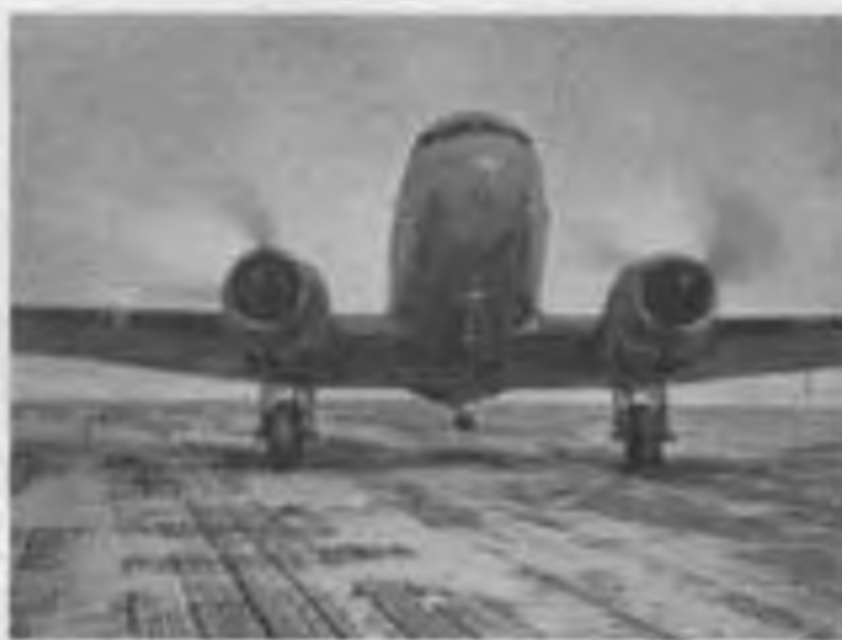
Figure 62. R4D (C-47) taxiing on PSP test strip. Note that very little snow is blown up by the propellers.
