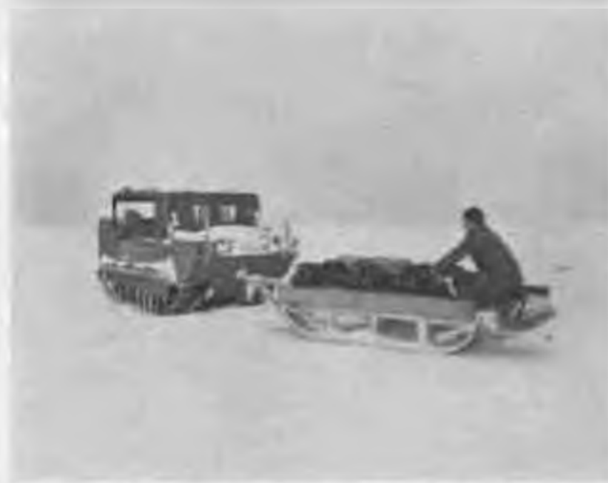
Figure 223. Weasel towing Army QM 1-ton sled.
