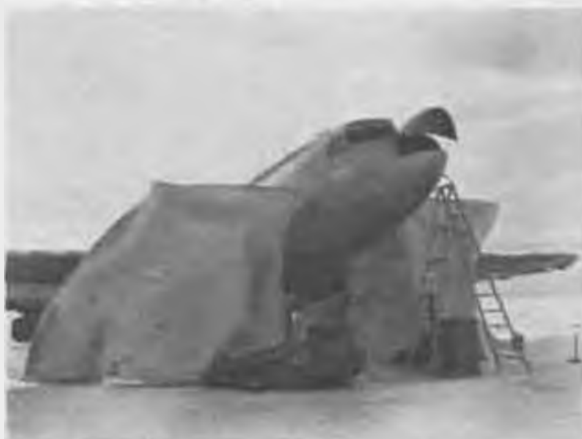
Figure 176. Improvised nose hangars for protection of aircraft maintenance personnel.
