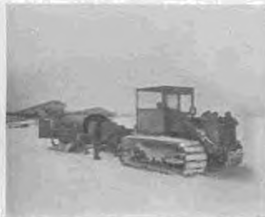
Figure 120. D-6 towing tank trailer.
