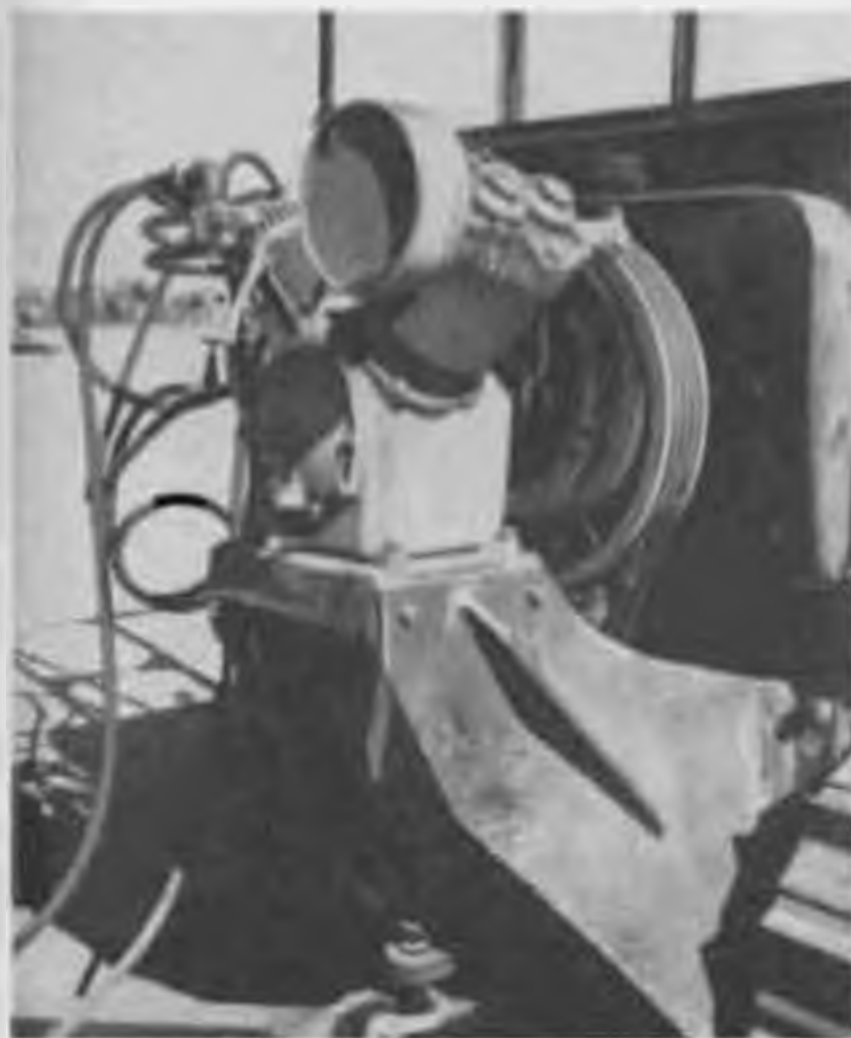
Figure 14. Compressor mounted (D-6 caterpillar tractor) for snow surface heater (40 cfm at 25 lb./sq. in.).
