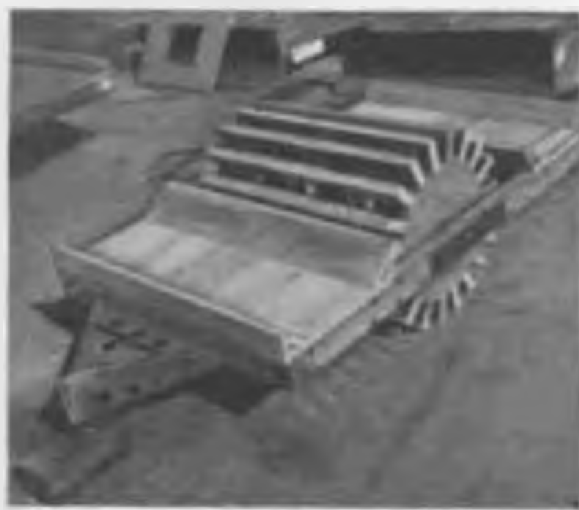
Figure 82. Open snow roller.
