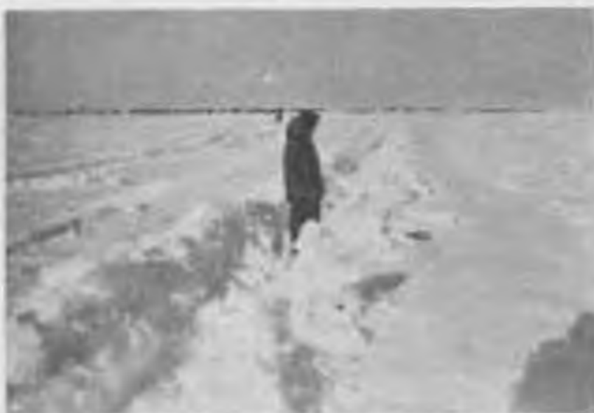
Figure 57. Track left after R4D (C-47), with wheels, had been towed from PSP test strip to ski runway No. 1. Tracks were almost waist deep in places.
