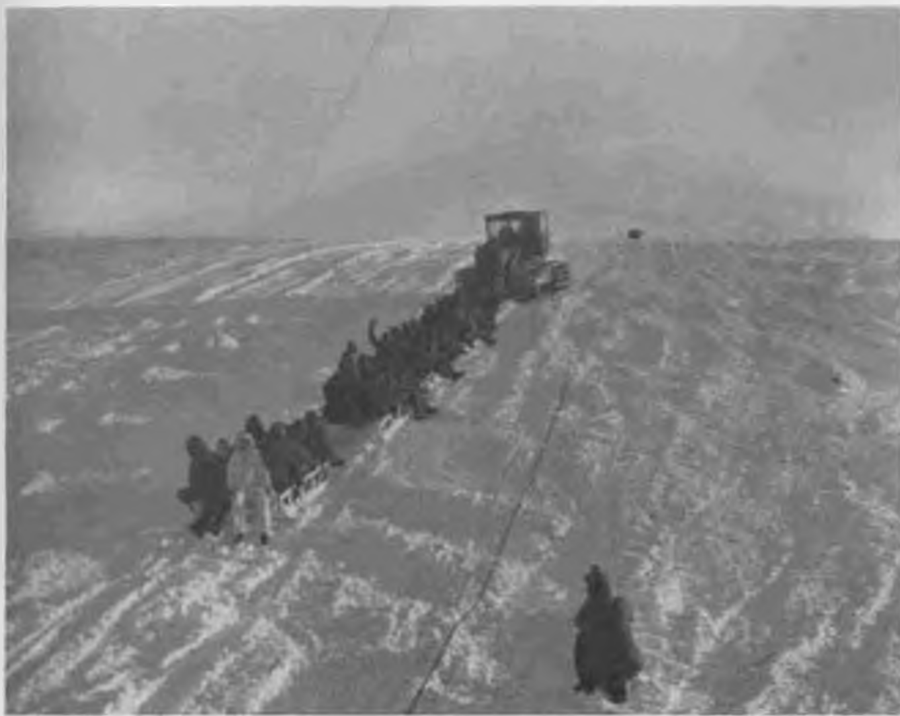
Figure 89. D-6 in reverse towing working party up barrier incline on five Army sleds.
