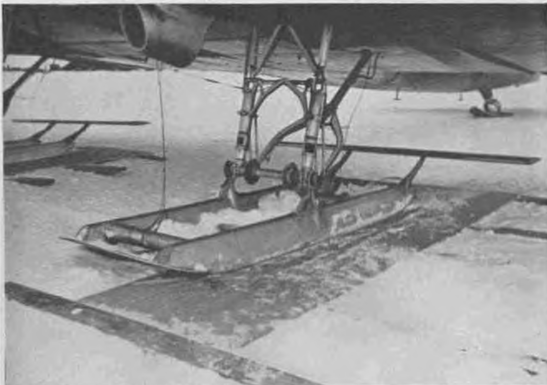
Figure 74. R4D (C-47) with skis, parked on plywood covered with Diesel oil to prevent skis from freezing to surface.
